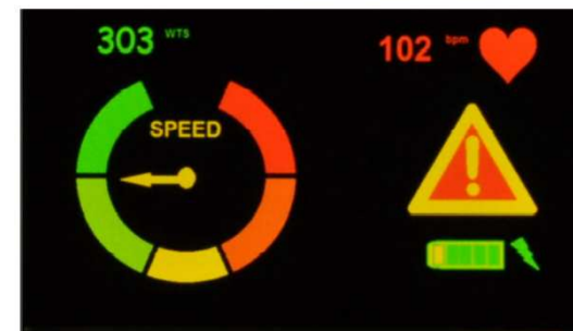
Photograph of the 2 color BY microdisplay demonstrator at 2000cd/m 2
